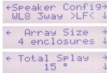
Figure 23 shows SC28 screen captures. The speaker configuration selected is WideLine-8, the array size is specified as four enclosures and the total splay is 15°. It's that easy, you don't have to do anything more.
