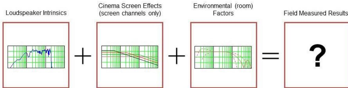
**1. Loudspeaker Intrinsic** – These refer to inherent characteristics of the loudspeaker and its components. These intrinsic are the result of natural physics; with current transducer technology, they are unavoidable, regardless of quality or cost. These intrinsic result in frequency response anomalies which cannot be corrected in the field, since their effects cannot be isolated from the other causal factors in the room.
