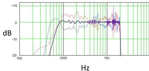
*A curve is generated representing the unaltered response of the loudspeaker (top, red line). Then, an inverse of that response is created using FIR filters (middle, blue line). When the two are combined, the result is a much flatter response (purple line, bottom).*
