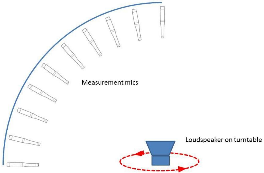
*A large number of specially-calibrated measurement microphones are mounted on a 90 degree arc. A loudspeaker is rotated on a turntable; at each degree of rotation, a series of measurements are made, resulting in a full 180 degree hemispheric series of measurements which capture the sound of the loudspeaker in every direction of its sound radiation.*
