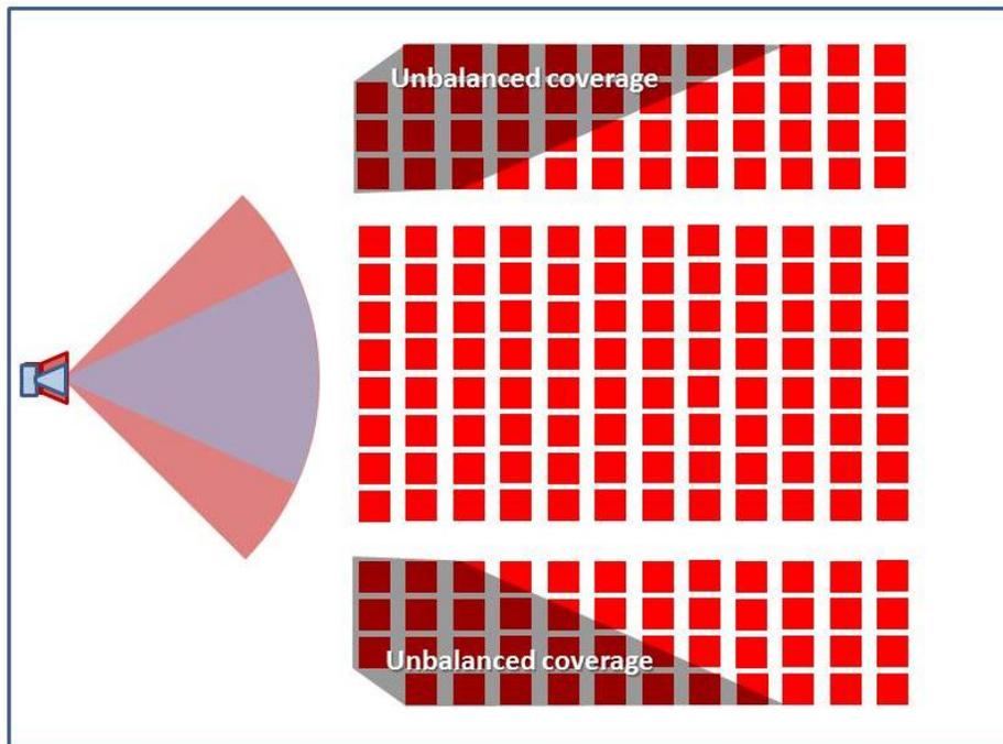
*A mismatch of the LF and HF horizontal coverage patterns at crossover can result in unbalanced coverage for up to 25% of the audience.*
