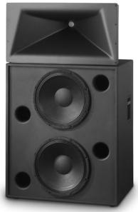
Developed specifically for the unique requirements of professional motion picture playback, the SC-322 extends QSC's commitment to the cinema market. As a member of the DCS Digital Cinema Speaker Series, the SC-322 is a 2-way, bi-amplified screen channel loudspeaker system comprised of two main units—the HF-63 high-frequency system and the LF-3215 low-frequency system.
