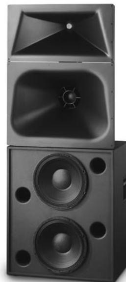
Developed specifically for the unique requirements of professional motion picture playback, the SC-423 extends QSC's commitment to the cinema market. As a member of the DCS Digital Cinema Speaker Series, the SC-423 is a 3-way, selectable bi or tri-amplified screen channel loudspeaker system comprised of two main units—the MH-1063 mid-high frequency system and the LF-4215 low-frequency system.
